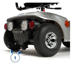
An anti-tipping (1) is fixed to the frame of the scooter on the rear side. It is not possible to remove these. The anti-tipping is there for your safety. It prevents the scooter from tipping over backward when you drive over small obstacles that do NOT exceed the maximum height as specified in §6.
