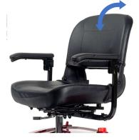
Push the backrest forward to fold the backrest to the front. Pull the backrest backwards to place the backrest in the upright position.
