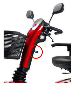
The steering unit can be adjusted to many different positions (stepless) to suit each driver.
